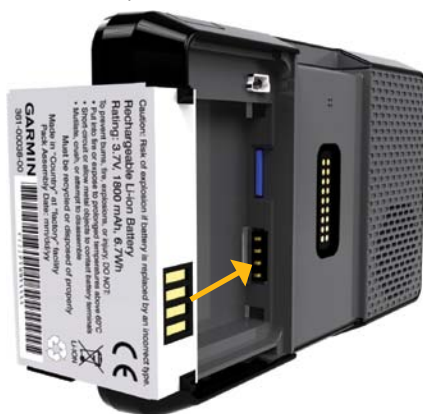
Installing the Battery
